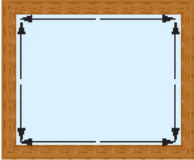
**Figure 3** The edges are then under stress to expand, this equals thermal stress. If this thermal stress meets or exceeds the breaking strength of the glass, thermal stress fracture of the glass pane occurs.
